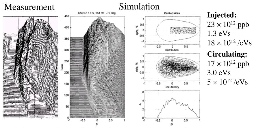
High B dot gives effective long. phase space painting. Injection period is approx. equal to synchrotron period.
